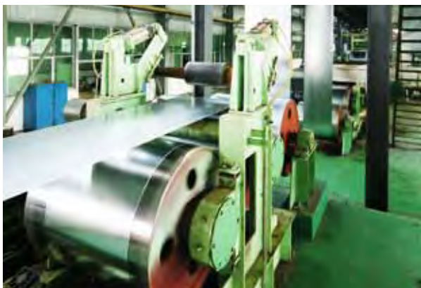
A steel coil galvanising production line
