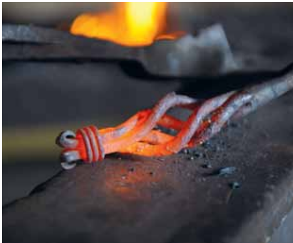
Iron is reheated to reduce its brittleness
