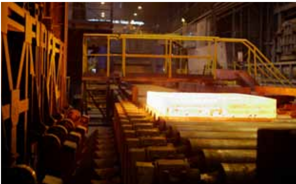
Hot rolling: A metal forming process in which metal stock is passed through a pair of rollers
