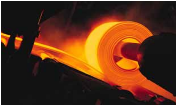
A large hot orange steel sheet being rolled in a steel mill
