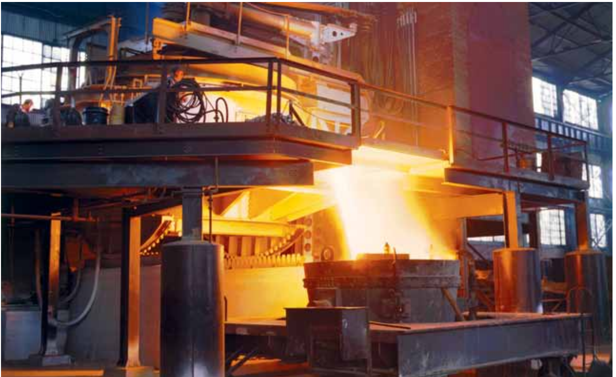
White-hot steel pours from a 35-tonne electric furnace, Allegheny Ludlum Steel Corp., Brackenridge, USA
